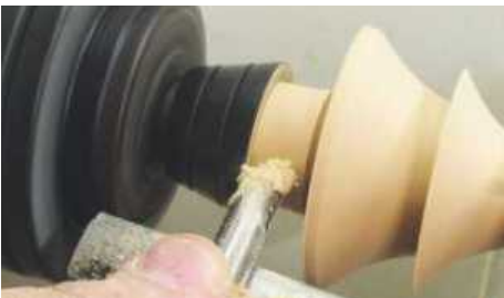
▲ Pic.7 Mask off the tree and spray or paint the base black or brown. Use the 10mm skew chisel to cut down the stem to the required diameter
